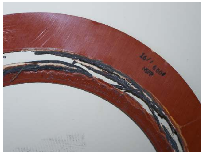
Figure 3. The tendency of phenolics to crack has eliminated them from flange isolation applications.
