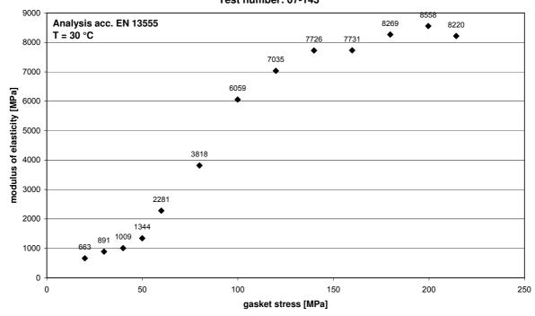
Compression test (RT) according EN 13555
