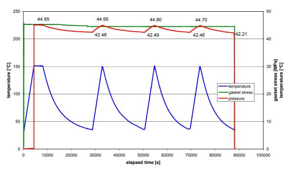
Shell cycle test at 150 °C according T-2.232686
