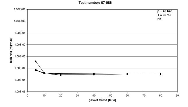
Leakage test according EN 13555
