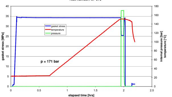
Hot Blow-Out Test HOBT Linebacker (Teflon) 133.2x77.9x3.96 mm Test number: 07-079
