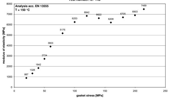
Compression test at 150 °C according EN 13555
