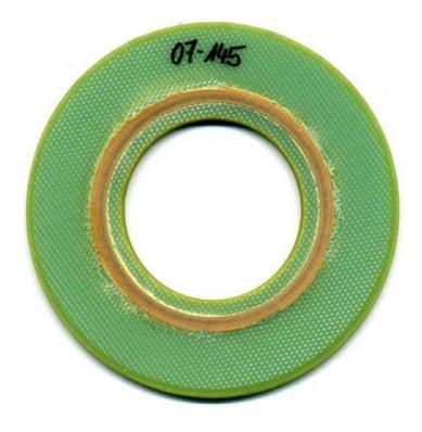
Compression test at 150°C (EN 13555)
