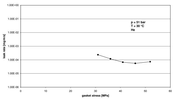
Shell leakage test (RT) according T-2.232686
