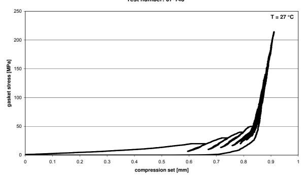
Modulus of elasticity Linebacker 91.7x43.4x4.10 mm Test number: 07-143
