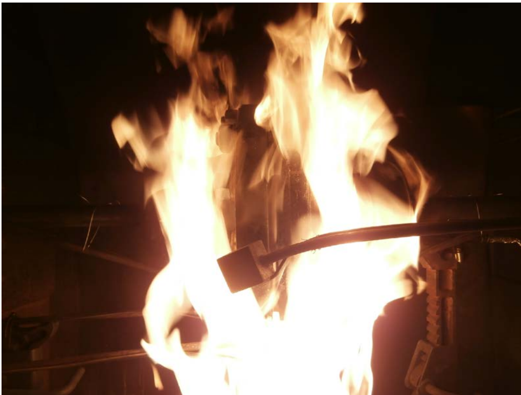
Test Gasket During Burn
