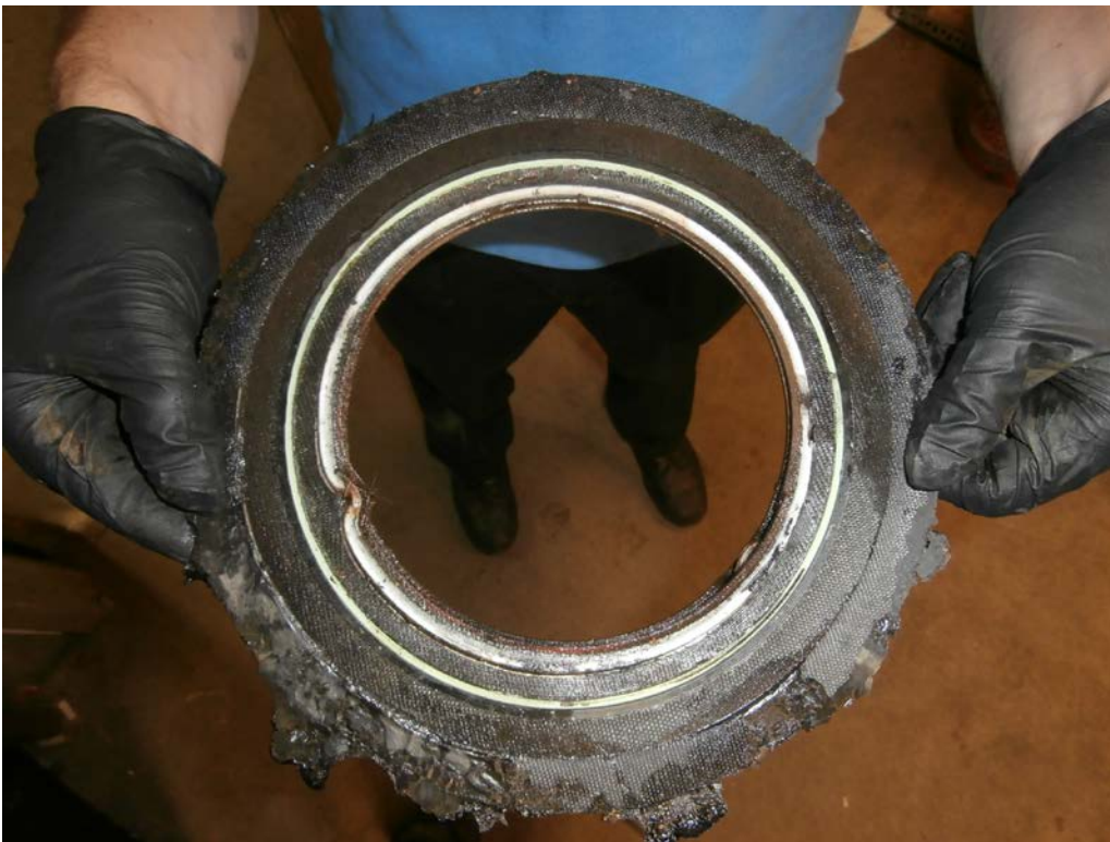
Test Gasket Post-Burn
