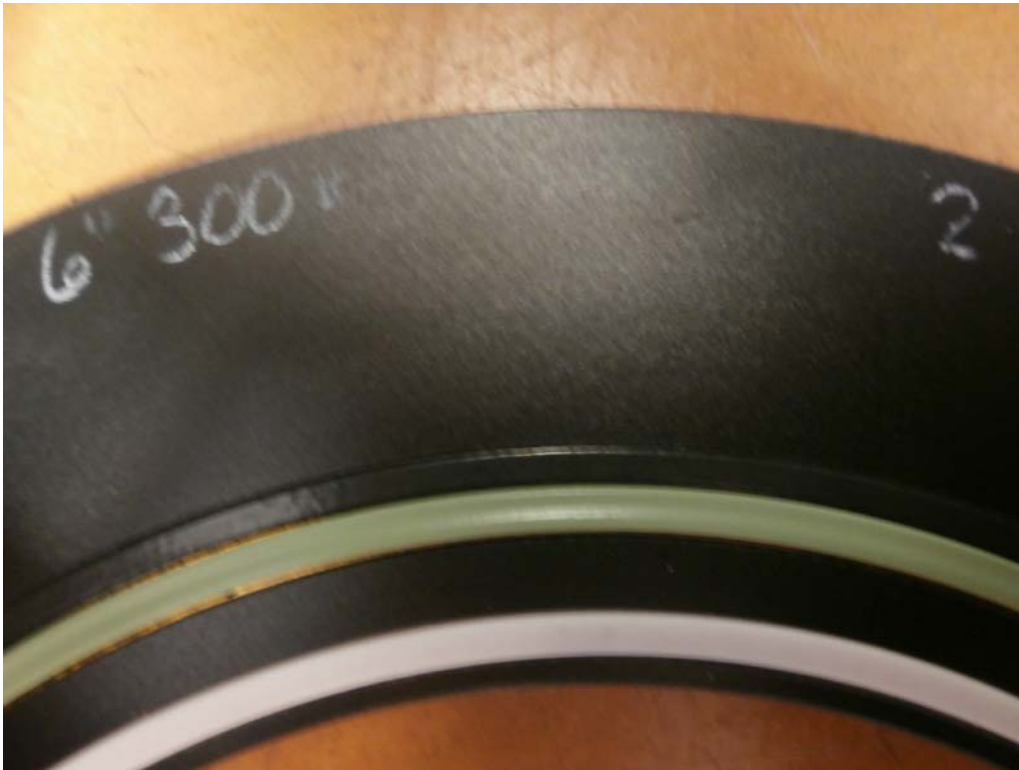
Test Gasket Prior to Burn
