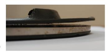
strength of the G10 or G11. High temperature, coupled with improper installation techniques or high pressures, can cause joint blowout.
