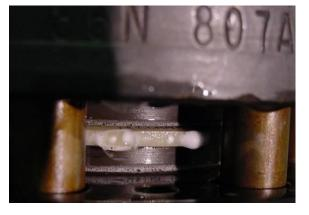
however media that permeated into the body of the gasket is able to potentially permeate from the inside diameter (ID) of the gasket to the outside diameter (OD) of the gasket causing emissions or visible leakage. Many users that use soapy water on the outside diameter of their plastic isolating gaskets have found bubbles forming from just this reason.
