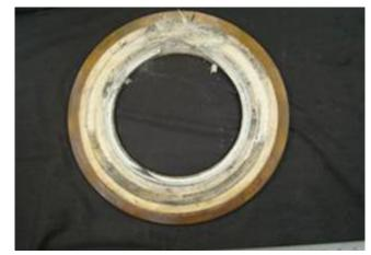
epoxy and this dramatically softens the laminate. With softening of the gasket and volume loss, blowout is a real danger.
