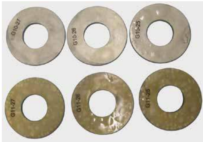
Chemical (H 2 S) attack on GRE isolation gasket
