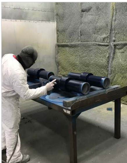
POLYURETHANE TOP COAT APPLICATION
