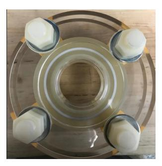
Image 3: A look down the flange bore with a properly sized gasket
