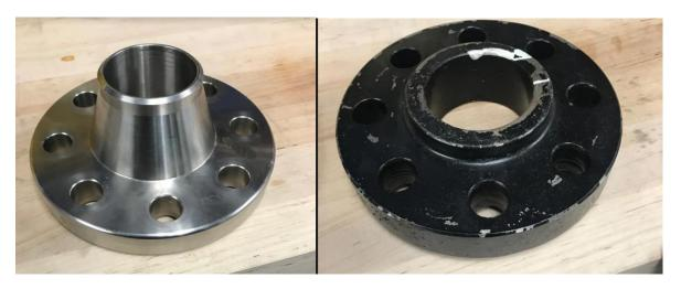
Image 1: Example of a Weld Neck Flange
