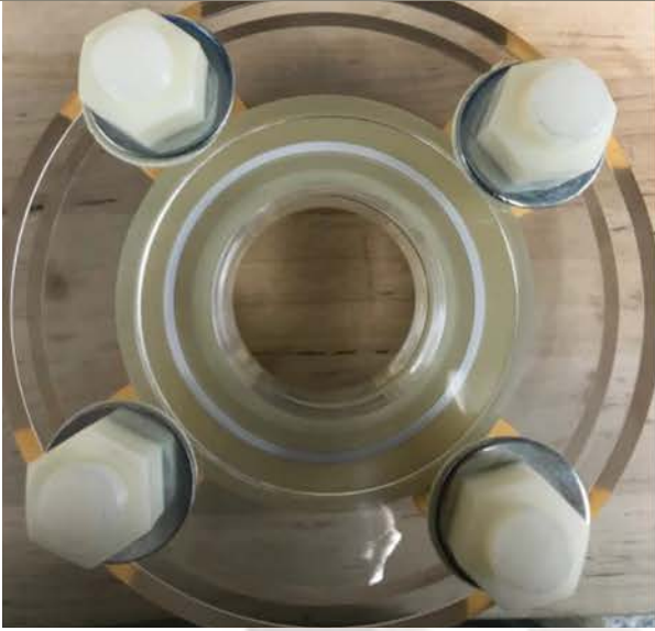
Image 3: A Look Down The Flange Bore With A Properly Sized Gasket
