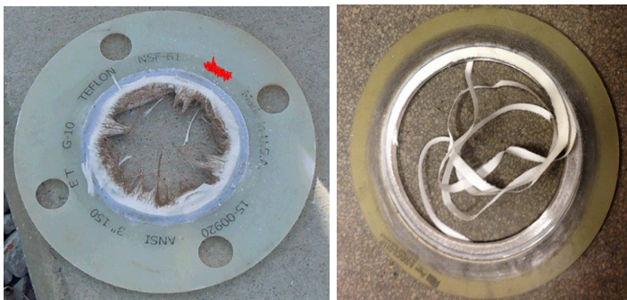
Images of isolation gaskets exposed to media and chemical attack.
