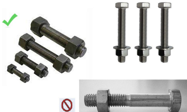
Use studs with two hex head nuts for flange isolation kits to ensure accurate torque and proper isolation. Avoid shoulder bolts, as their unthreaded sections prevent sleeves from fitting, rendering the kit ineffective.
